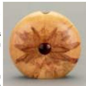
A 2" slice cut horizontally from a log was mounted on a vacuum chuck and rounded off on both sides (contour gauge) to form a discus. The bottom was sanded flat with a disc sander and 180 degrees from this base, a hole was drilled to accept a glass vase insert. To complete the allusion, two 1" stemmed bloodwood buttons, to resemble the insipient black hole, were turned and glued into holes drilled into the center of each face. It was finished in the usual way.
