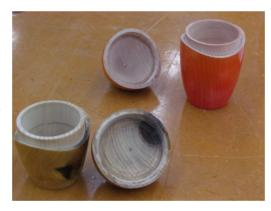
Hollow out the lid slightly with a bowl gouge, leaving a 1/8" flat area.
